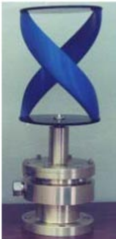
Double-Helix Turbine (for underwater installation)
