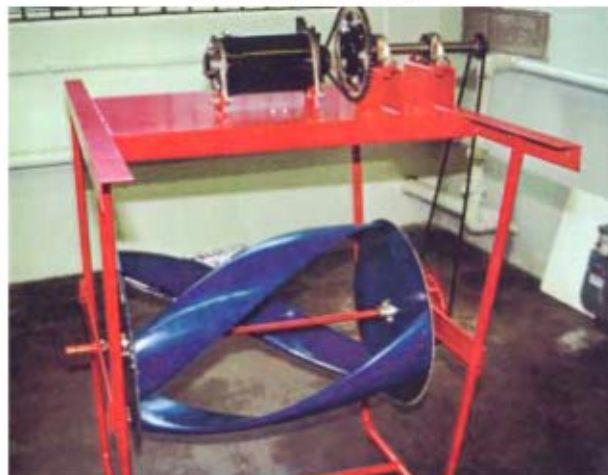
Power systems for free flows with different helical turbines
